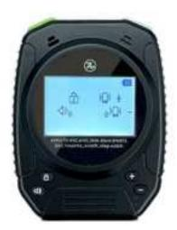
Under non-timed state, press the volume button for 2 seconds to quickly enter the interface for checking group scores.
