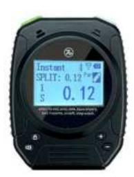
Under non-timed state, press "-" button for 2 seconds to quickly begin countdown function.
