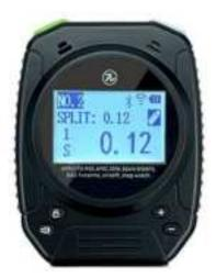
Under non-timed state, press the "+" button for 2 seconds to quickly start/stop "PAR" mode.
