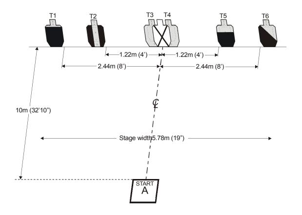
**SETUP NOTES:** Set paper targets to 1.52m (5 feet) to the top of targets. Area A is 0.92m (3') by 0.92m (3').T1 hard cover is from top of A zone down. T2 hard cover is from perforation of A zone outward from top to bottom on both sides of A zone. T5 hard cover cuts through center of A zone. T6 hard cover runs diagonal from top left notch downward to top bottom notch. T3 and T4 are butted edge to edge, the penalty target is then centered on them. Center of the penalty target is on center line.
