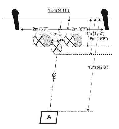
Setup notes: Set paper targets at 1.52m (5 feet) to the top of targets. Areas A is 0.92m (3') by 0.92m (3').
