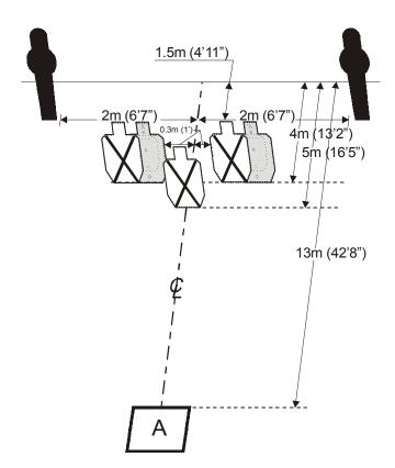
Setup notes: Set paper targets at 1.52m (5 feet) to the top of targets. Areas A is 0.92m (3') by 0.92m (3').
